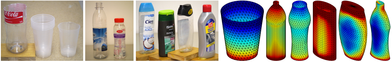
Fig. 2: Artificial dataset (right) built according to real objects (left). Coloring represents local stiffness, see text.
